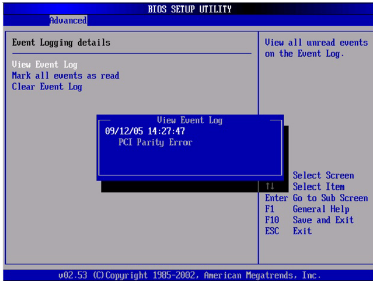
FIGURE E-4 Sample DMI Log Screen, PCI Parity Error
