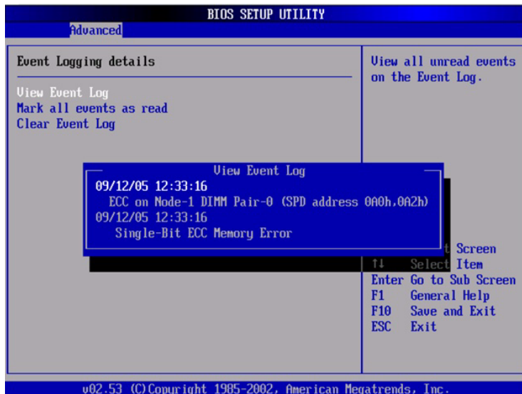
FIGURE E-2 Sample DMI Log Screen, Correctable Error
