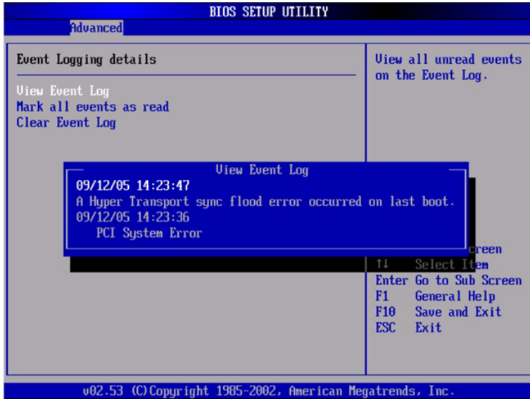
FIGURE E-6 Sample DMI Log Screen, System Error Listed
