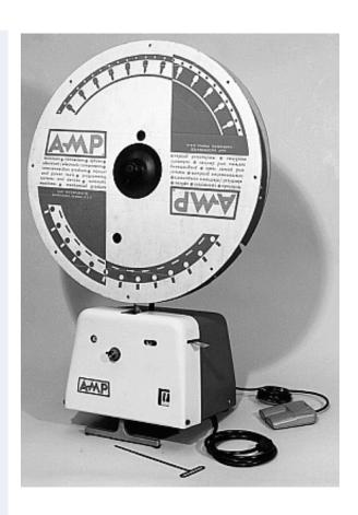
AMP-TAPEMATIC Stripper/Crimper Machine No. 599406-7
