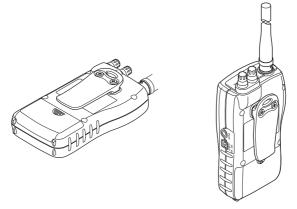
To make your scanner easier to carry when you are on the go, use the supplied belt clip. Use a Phillips screwdriver and the supplied screws to attach the clip to the scanner.
