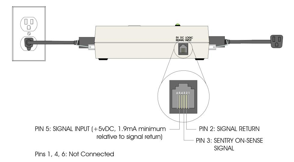
Always-On IPMs (normally-closed relays): +5vDC relative to signal return turns power off
